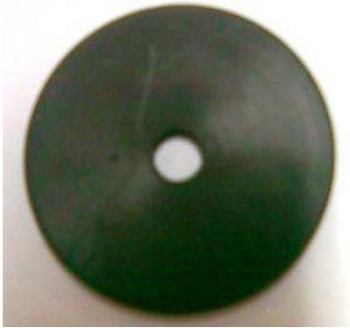
Fig. 1: MREs sample with 50 wt. % Carbonyl-iron
