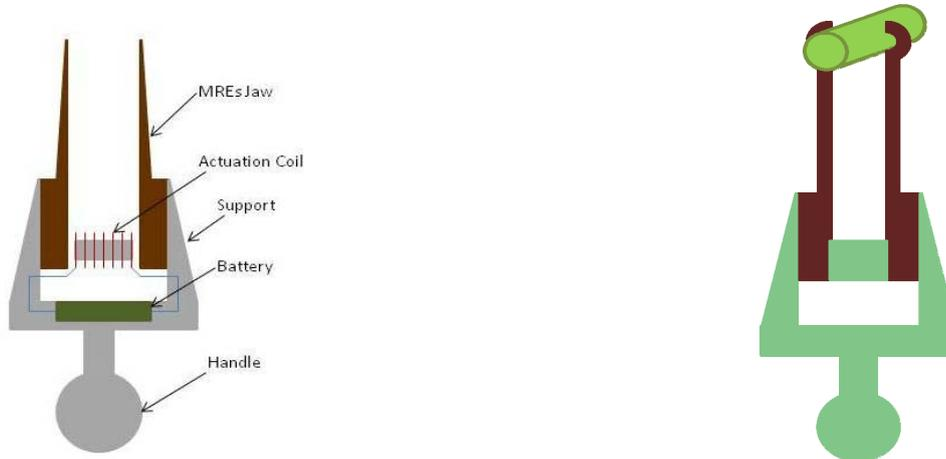
Fig. 10: Schamatic diagram of a simple MREs miniature gripper. Fig. 11: Schamatic diagram of MREs hooke-style miniature gripper.
