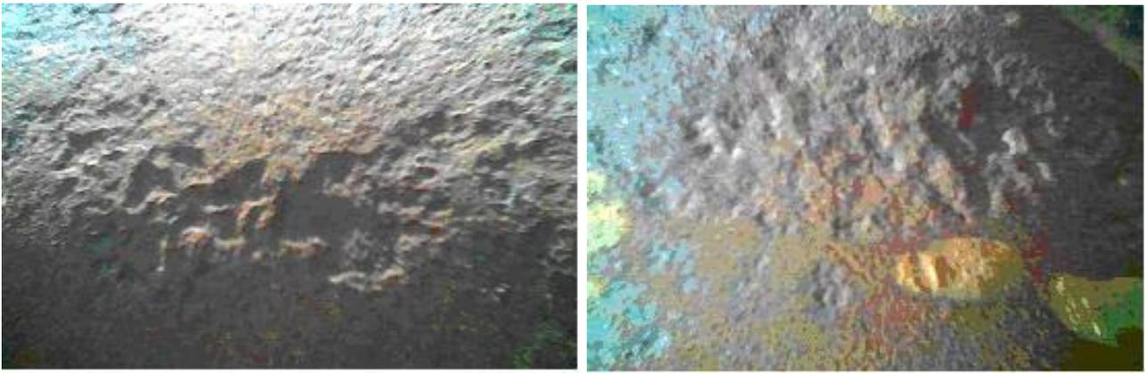
Fig. 1-2: Corrosion under insulation in maroon desalting plants
