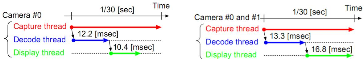
Fig. 3: (Left) Running time of each thread with one camera, (Right) Running time of each thread with two cameras.
