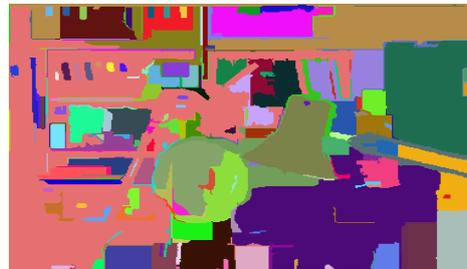
Fig 3(b) Bilateral filtered Graph-based Segmented Right Image
