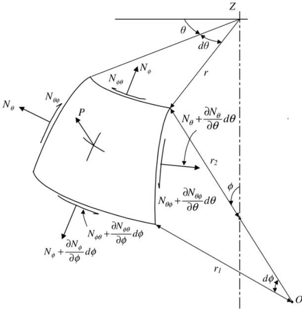
Fig.1. Direct and Shear Stress Resultant in Hemispherical Dome [9]
