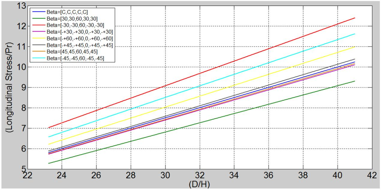
Fig.7. Effect of the Fiber Angle Orientation on the Behavior of Laminated Hemispherical GRP Dome Internally Pressurized
