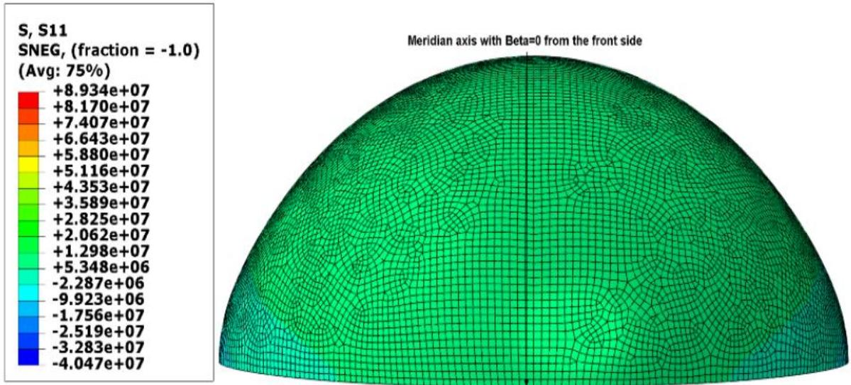
Fig.5. Front View of Hemispherical GRP Dome,  $P_r=1$ [MPa],  $(D/H)=38.037$ ,  $k=1$  and  $t=0.01$ [m] after Deformation
