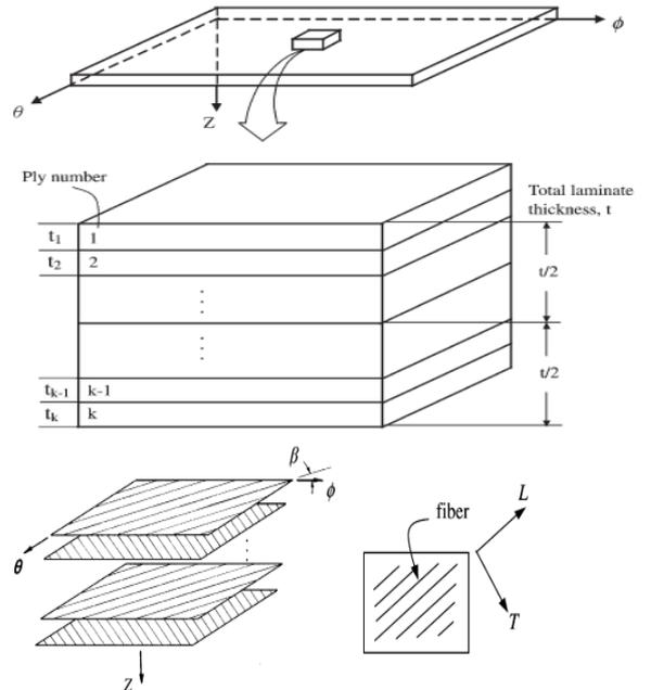
Fig.2. Schematic of a Lamination Geometry with Winding angle of Fibers [9]
