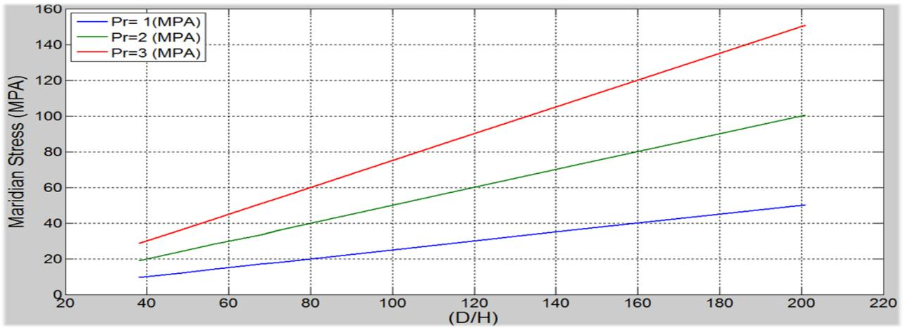
Fig.6. Effect of Internal Pressure on Meridian Stress in laminated Hemispherical GRP Dome
