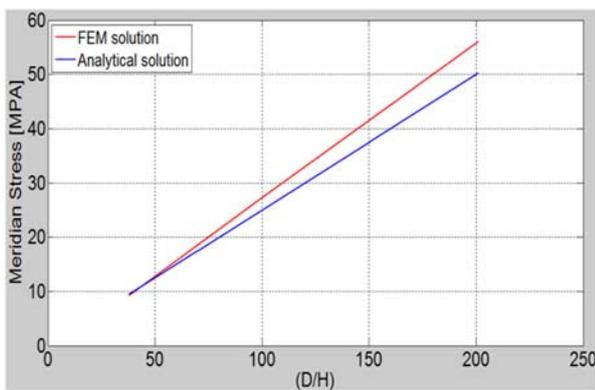
Fig.3. Comparison of the FEM and Analytical Meridian Stress Results in the Hemispherical GRP Dome at Pr=1MPa
