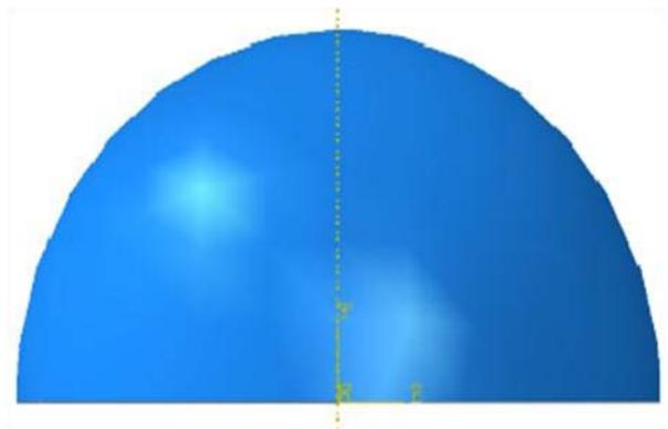
Fig.4. Front View of Hemispherical GRP dome, Pr=1[MPa], (D/H) =38.037, k=1 and t=0.01[m] before Deformation
