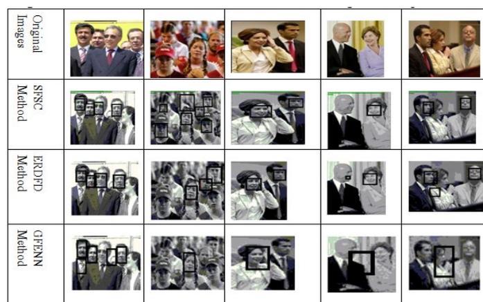
Fig. 3: Face Detection results of the three methods for the images of multiple faces
