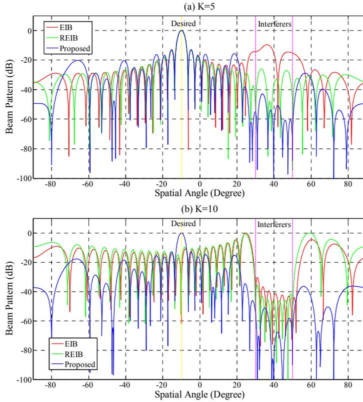
Fig. 3: Beam patterns obtained with  $\theta_s = 3.2^\circ$  and  $N_s = \infty$ . (a)  $K = 5$ ; (b)  $K = 10$ .
