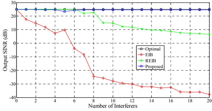
Fig. 2: Output SINR performance versus number of interferers ( $K$ ).  $\theta_s = 3.2^\circ$  and  $N_s = \infty$ .
