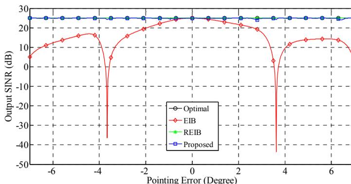
Fig. 1: Output SINR performance versus pointing error ( $\theta_s$ ).  $K = 3$  and  $N_s = \infty$ .
