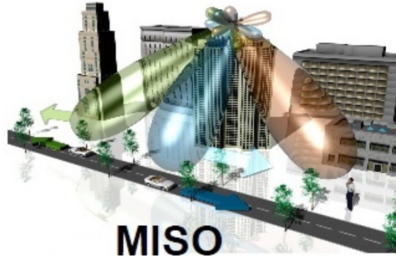
Fig. 3: Transmit beam-forming depending on the angle of each user (Rank 1 CLSM).
