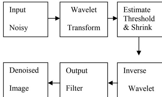
Fig. 2 Procedure to denoise an ultrasound image
