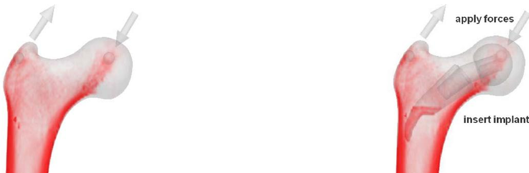
Fig. 1. Von Mises stresses (calculated for polynomial degree of 6) of a healthy bone (left) and after a virtual surgery (right), under load exerted at the femur's head and the greater trochanter; darker colour refers to the regions with higher stress magnitude, thus, provides overview of how the implant changes the stress distribution in the surrounding bone tissue.
