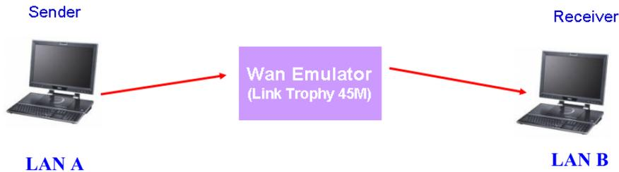
Fig. 2. Experiment setup for the wired environment without traffic and with Wireshark.
