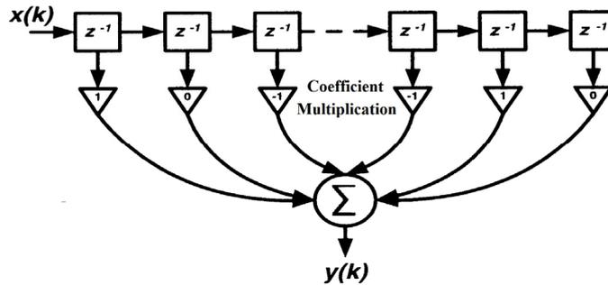
Fig. 1: Block Diagram of a Ternary FIR Filter (from [1]).
