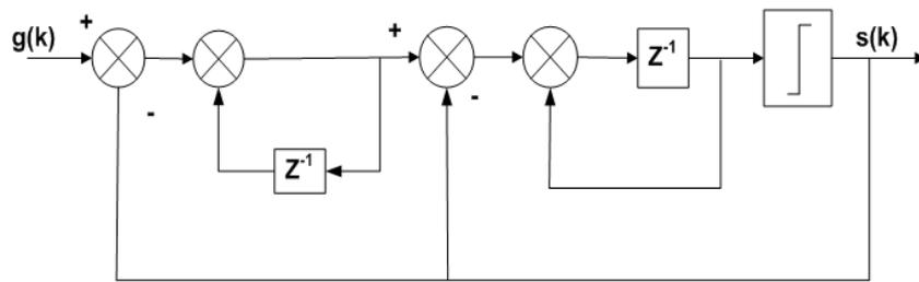
Fig.3: Block Diagram of a Second-order  $\Sigma\Delta$  Modulator.
