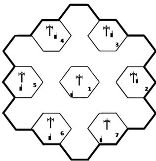
Fig. 1: Arrangement of mobile stations and BTSs
