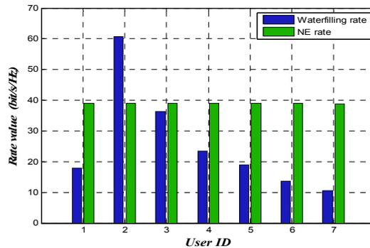
Fig. 5: Comparison between total data rate in non-cooperative power control game at NE and WF method. The NE rate is fair (equal for all users).
